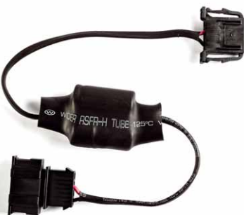
In the T5, the woofer needs this low pass crossover
