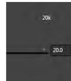
This indicator allows you to see the current frequency that has been selected with the corresponding channel in the crossover adjustment tool. In addition to making frequency adjustments with the frequency slider you may also click on this readout display box and manually enter the desired frequency for the channels that you are currently adjusting.
