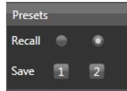
The Preset function allows you to store two different settings at your DSP amplifier. Both settings can later be switched by the user. To do the selection connect the “user program switch”(14) to gnd. The preset 2 will then be active. Open the switch will result to switch back to Preset 1.
