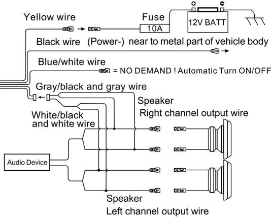
Wiring Diagram1 (High level input)
