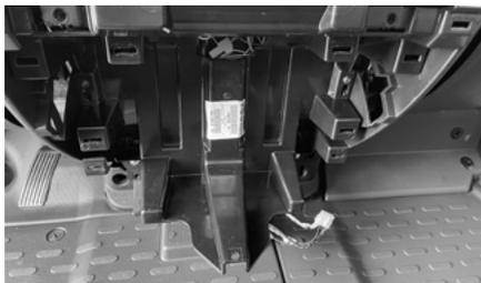
**Step 14):** Then insert the cup holder. Make sure that all clips engage properly, broken clips/metal clamps should be replaced. Make sure that no connection cables are crushed or damaged when inserting the beverage holder.
