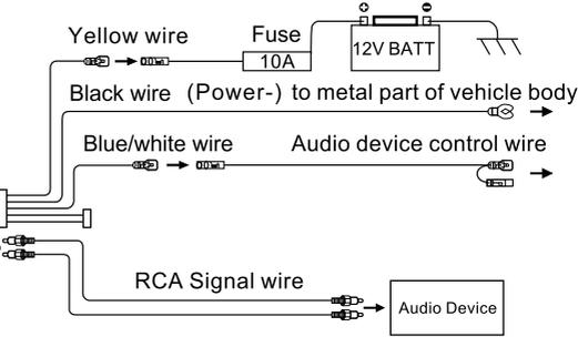
Wiring Diagram2 (Low level 'RCA' input)
